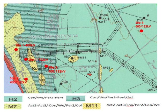
Figure 5: Geotechnical Series Map - Koeberg Substation
